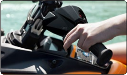
iBR - Intelligent Brake & Reverse Exclusive to Sea-Doo® models, iBR stops the watercraft sooner and provides more control and maneuverability at low speeds and in reverse.
